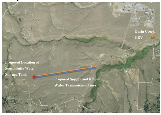
Only a storage tank and associated transmission piping installations are included in the Groundwater Restoration Plan. These components are a requirement to restore water service to the South Side Pressure Zone (South Butte) and are not dependent upon other improvements. Moreover, they will not be sacrificed when other improvements are made to the system in future years.
