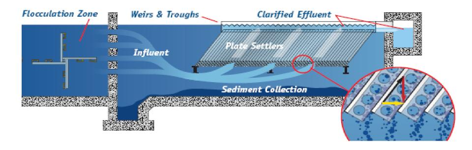
Enhanced coagulation is the process of adding coagulants that targets high removal of TOC by binding the dissolved organic carbon into a flocculant which settles and can be removed from the raw water supply.
