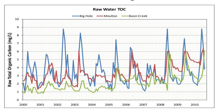
There has been a trend of increasing Total Organic Carbon TOC concentrations in the three raw water sources. When these TOCs come in contact with chlorine for disinfection, secondary disinfection byproducts (DBP's) are formed. TOC removal requires enhanced pretreatment of the raw water prior to chlorine contact to minimize the DBP formation.
