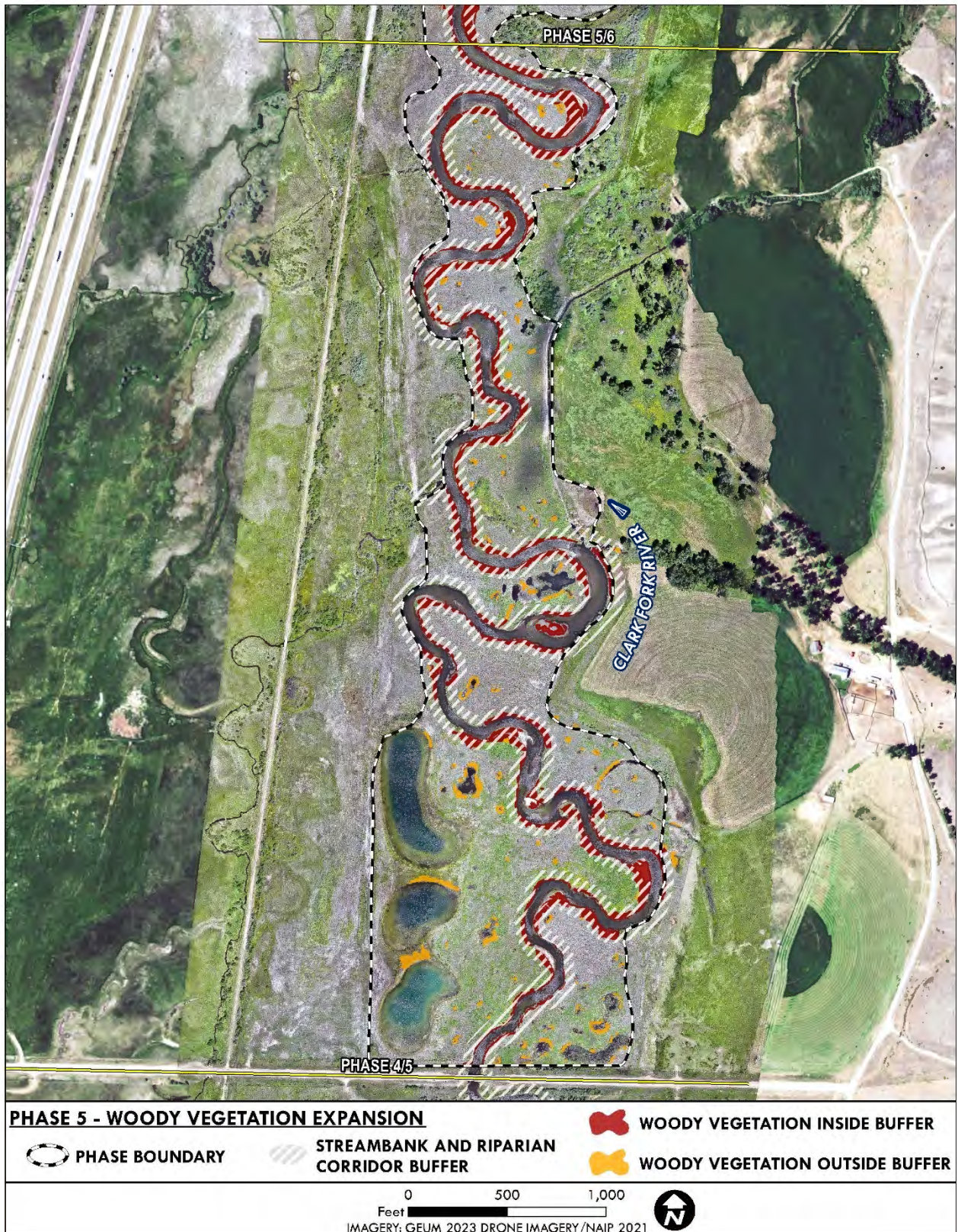
Figure 17. Estimated woody vegetation cover within the 50-foot Streambank and Riparian Corridor Buffer Zone and outside this zone but within construction limits for Phase 5.
