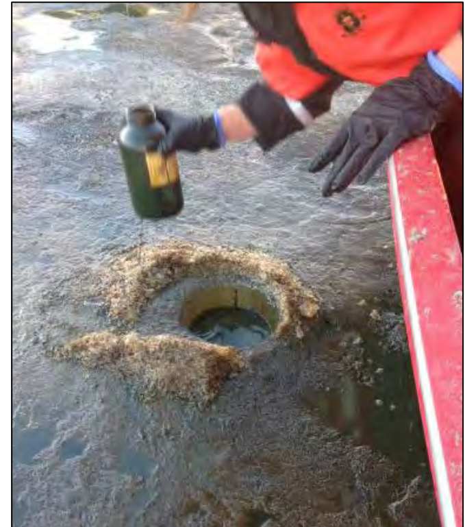
U.S. Coast Guard collecting water samples through holes cored in the ice on the Yellowstone River - January 26 Source: Weston Solutions, 2015
