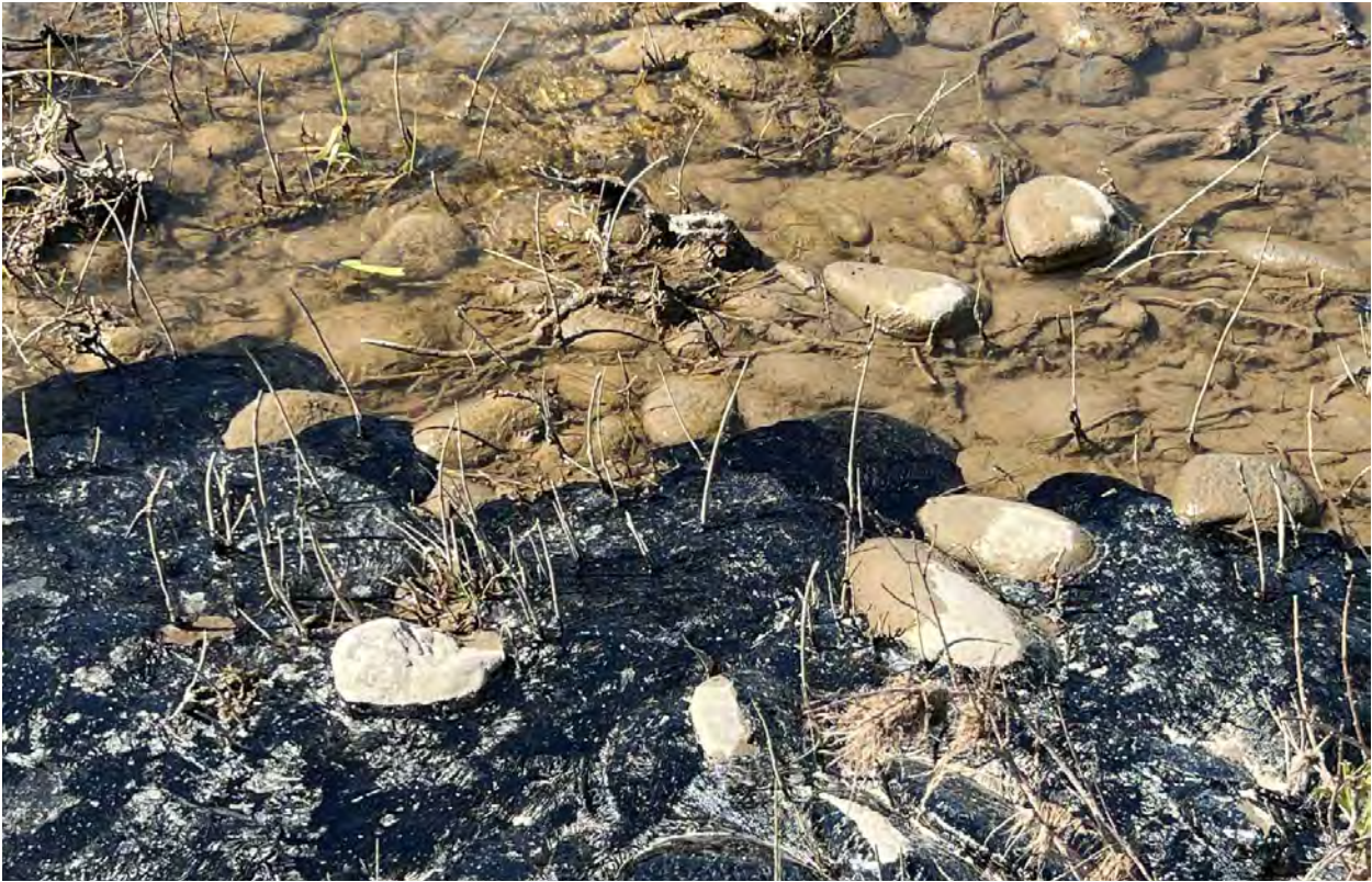
Exhibit 2-1. Asphalt deposits along shoreline. Photos taken approximately 1.5 miles downstream of the train derailment site, on the lee side of an island.
