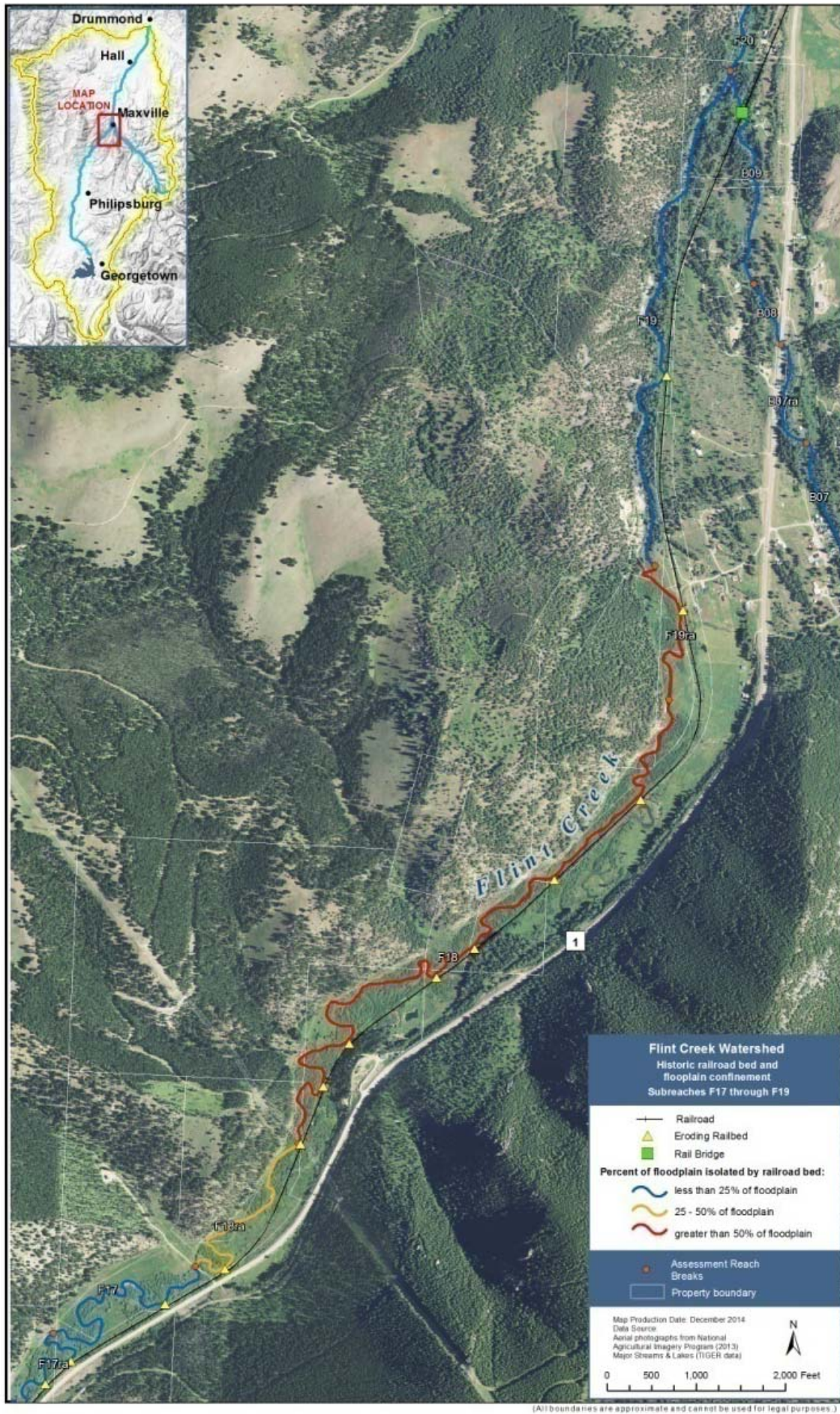
Figure 19. Railroad constriction of stream between F17 – F19
