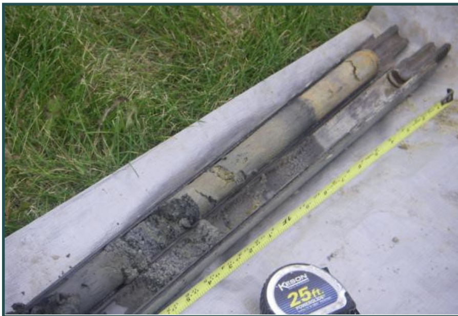
2009 MBMG Parrot Investigation—core sample containing tailings
