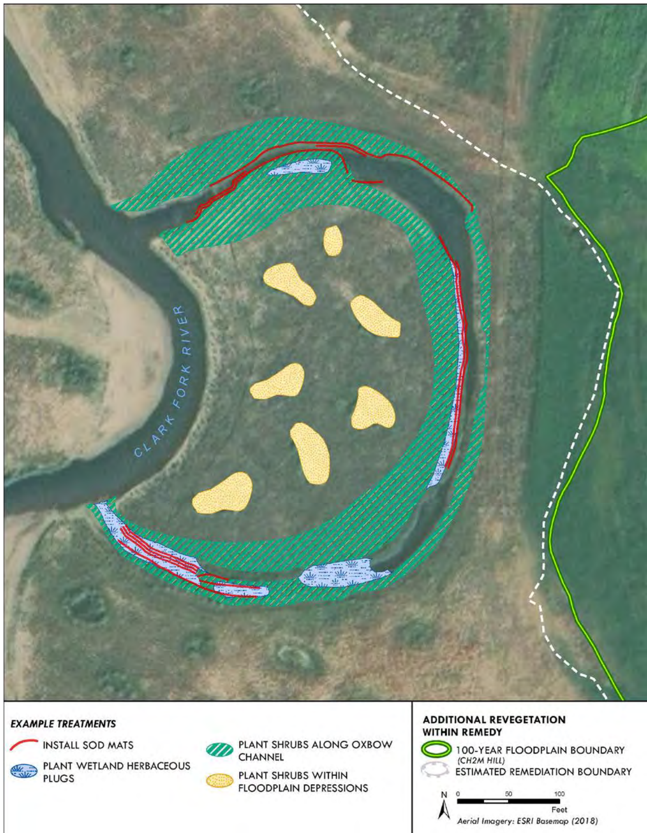
Figure 6. Example treatments that may apply within the Additional Revegetation (Within Remedy) restoration action.
