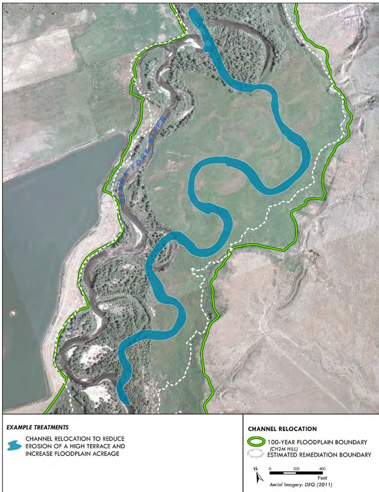
Figure 12. Example of the Channel Relocation restoration action.
