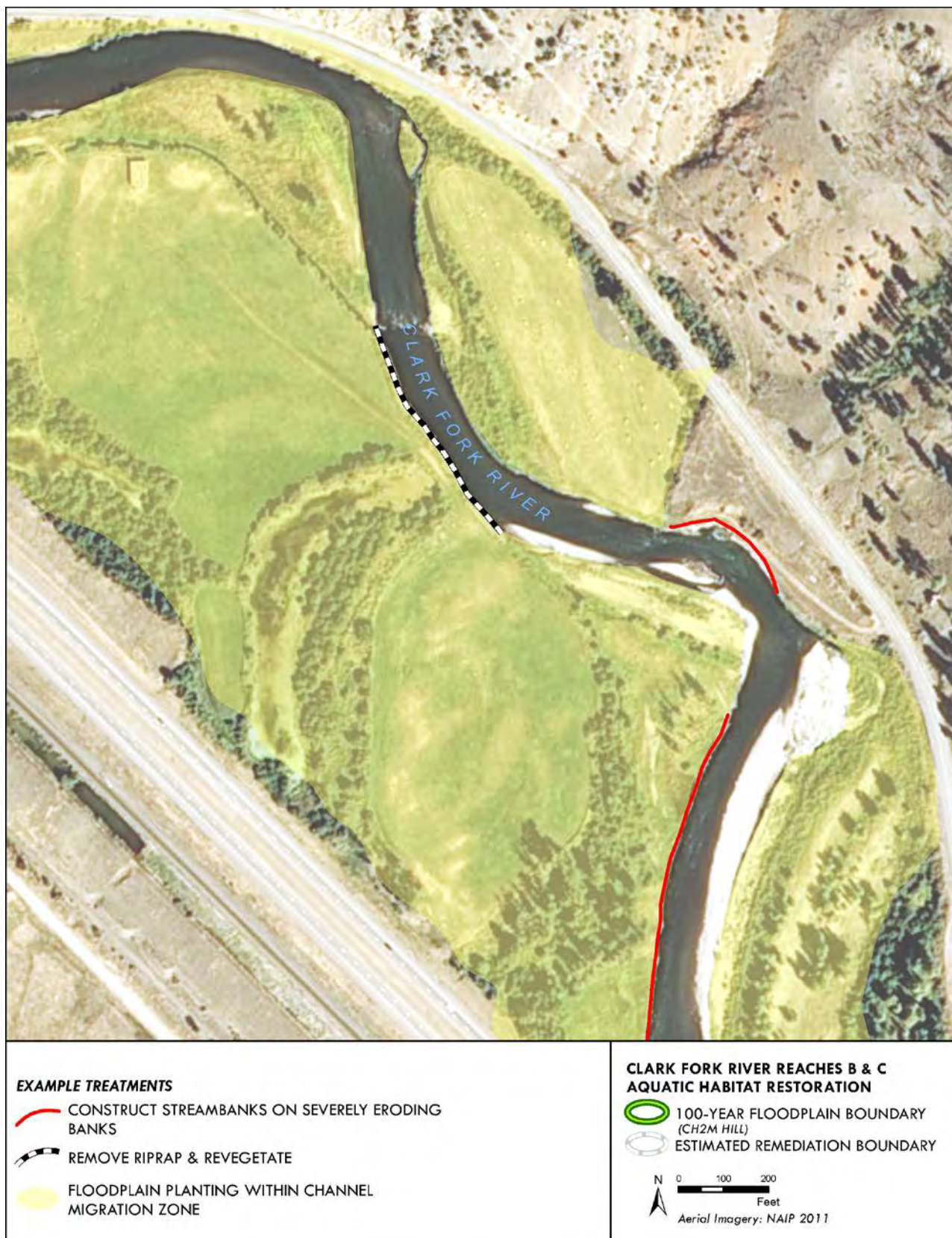
Figure 14. Example of treatments that may apply within the Clark Fork River Reaches B and C Aquatic Habitat restoration action.
