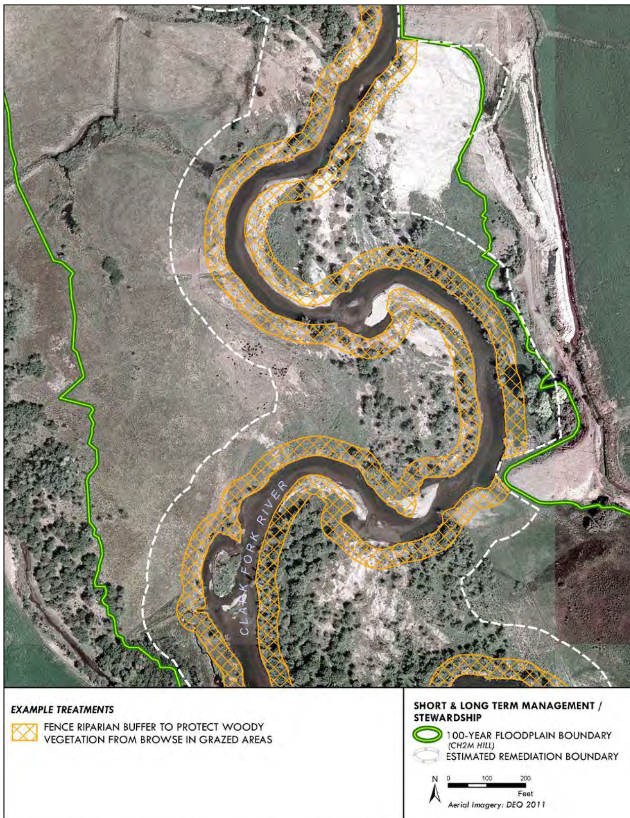
Figure 9. Example treatment that may apply within the Short and Long term Management/Stewardship restoration action.
